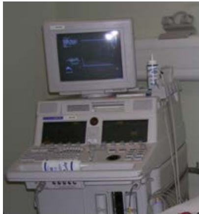
Fig. 1: Ultrasound system utilized for measuring diameter of the BA and recording the BA images
